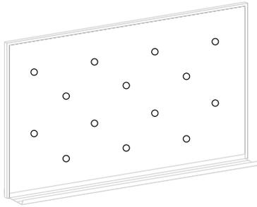
Prepare the surface of the existing board by thoroughly cleaning it of dirt, dust, or grease. Apply construction adhesive to the surface of the existing board in golf-ball size amounts every 16" in height and every 24" in length.
