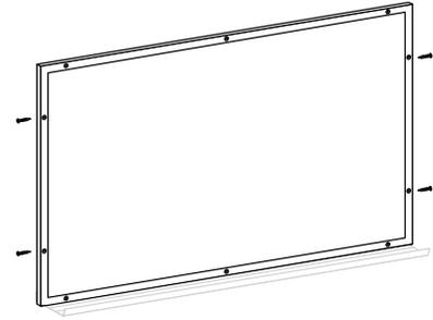
Install the self-tapping screws (supplied with the board) through the pre-drilled holes in the trim. Clean the board thoroughly before using. See markerboard care and maintenance instructions.
