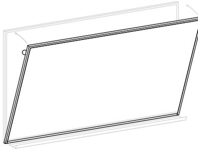
Position the new board carefully over existing board, and press firmly in the locations of the adhesive.
